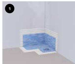
1 Clean the surface. Apply Foil Seal to the corner and install Inner/Outer Corners. In the case of an absorbent surface, SCHÖNOX WSA can be used instead. Press hard.
