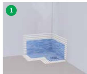
Clean the surface. Apply Foil Seal to the corner and install Inner/Outer Corners. In the case of an absorbent surface, WetStop adhesive can be used instead. Press hard.
